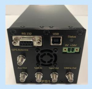
RFS1B with integrated GNSS receiver
