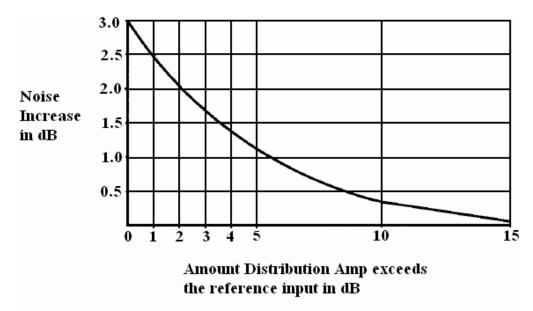
The DistAmp must ideally exceed the reference sources phase noise by at least 10 dB. Referring to the above graph, 10 dB (on the X axis) corresponds to 0.4 on the Y axis. So, if the DistAmp's phase noise is 10 dB better than the reference, and the reference is connected to this DistAmp, the DistAmp will add 0.4 dB to the references phase noise. Thus, ideally the DistAmp must be 15 dB better than the reference phase noise.
