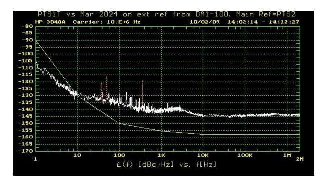
See how the phase noise at 1 Hz offset is 26 dB better and 10 dB better at 10 Hz offset. This amazing improvement is due to the Marconi 2024 now having an ultra-low noise reference. This phase noise will also improve the Marconi 2024's Allan variance.
