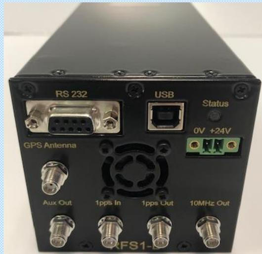
**RFS1B with integrated GNSS receiver**
