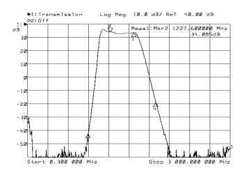
The above picture shows the GPS35-BNC frequency response from 300 kHz to 3 GHz. Ultimate rejection is typically > 80 dB
