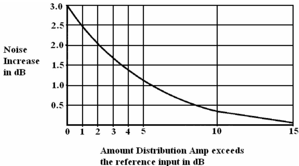
The DistAmp must ideally exceed the reference sources phase noise by at least 10 dB. Referring to the above graph, 10 dB (on the X axis) corresponds to 0.4 on the Y axis. So, if the DistAmp's phase noise is 10 dB better than the reference, and the reference is connected to this DistAmp, the DistAmp will add 0.4 dB to the references phase noise. Thus, ideally the DistAmp must be 15 dB better than the reference phase noise.
