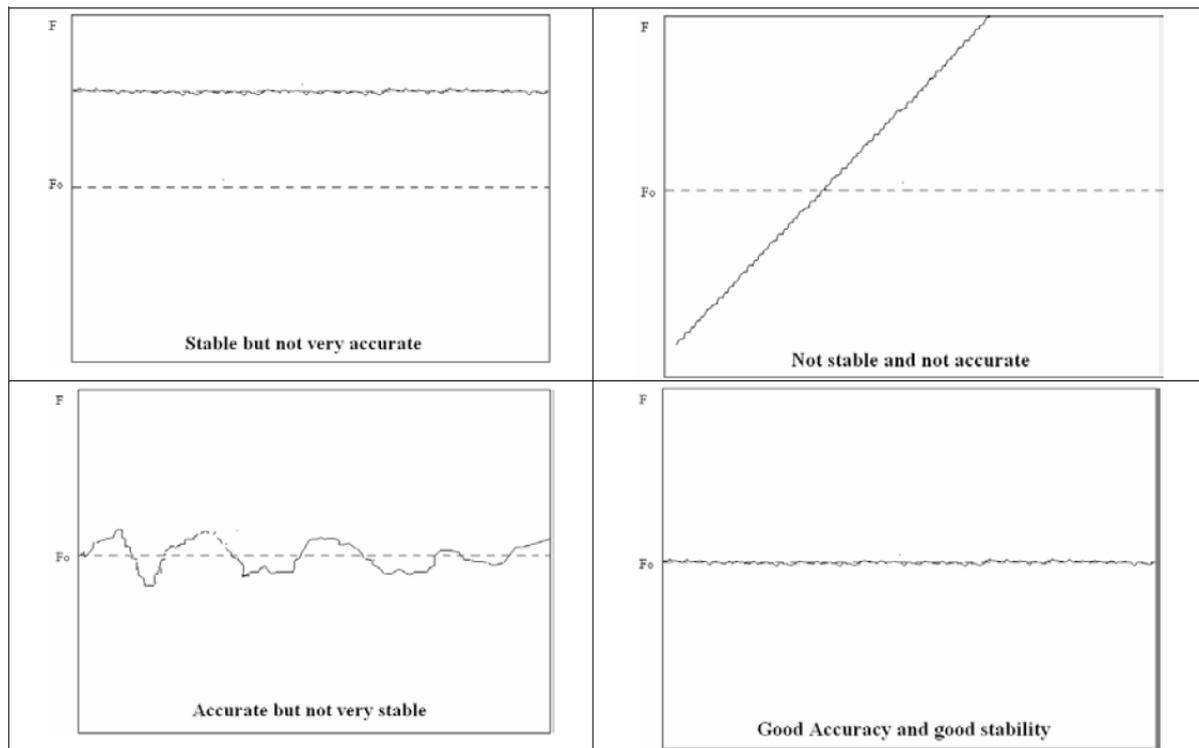
Ideally we want an oscillator that has a good Allan Deviation and is also accurate as shown in the bottom right graph.
