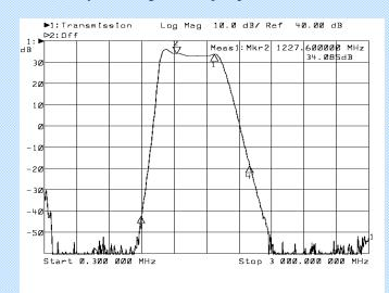
The above picture shows the GPS35-BNC frequency response from 300 kHz to 3 GHz. Ultimate rejection is typically > 80 dB
