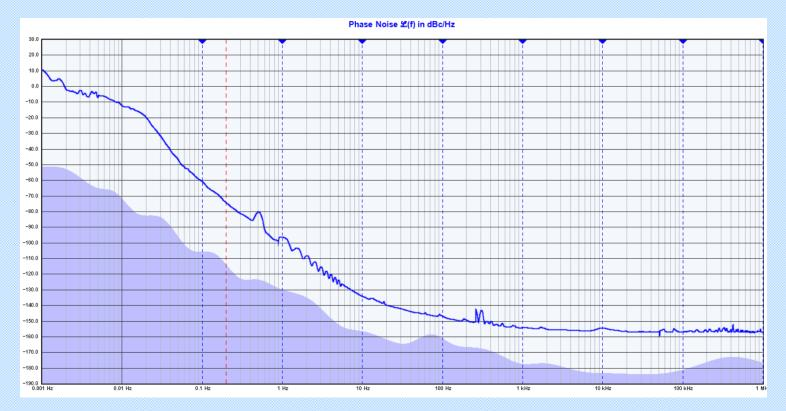
Above plot shows the typical Phase Noise. Below plot is the Allan deviation
